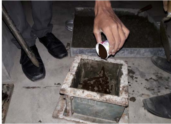
Fig. 3. Mixing bitumen in the mould.
